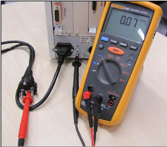
Figure 6: Measuring ground wire resistance
