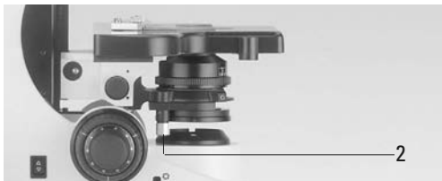
Fig. 23 Assembling the polarizer holder 1 Clamping screw
