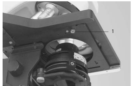
Fig. 6 Assembling the coaxial pinion
