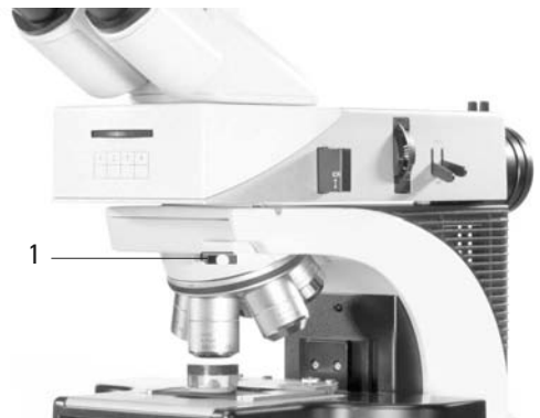
Fig. 57 Objective prism with setscrew
