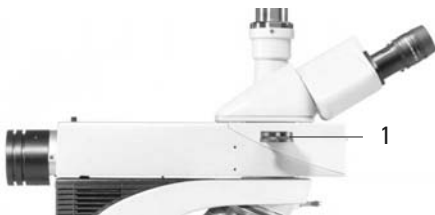
Fig. 24 Assembling the analyzer 1 Analyzer
