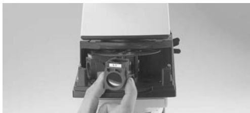
Fig. 22 Inserting the filter cube
