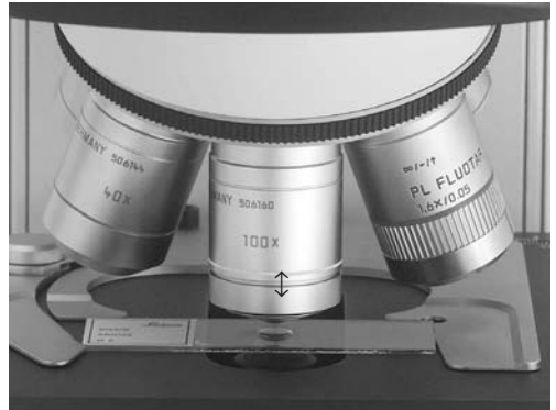
Fig. 51 Immersion objective, locked
