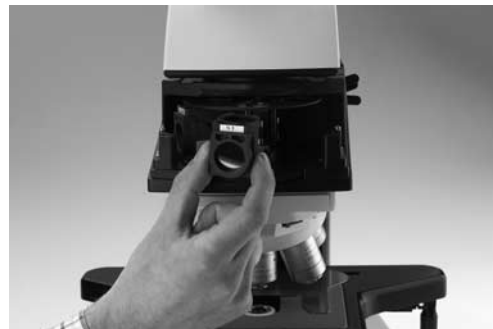
Fig. 25 Mounting the Filter cube
