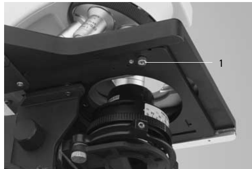
Fig. 7 Coaxial pinion installation 1 Mounting screw for coaxial pinion
