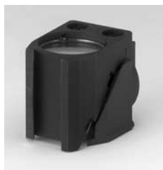
Fig. 22 Filter cube back side
